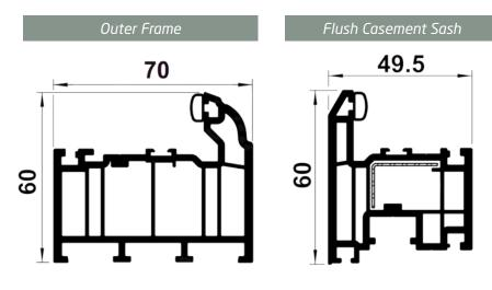
The flush casement window measures 70mm from back to front, with a sash width of 60mm and the option of a deep bottom rail of 90mm
